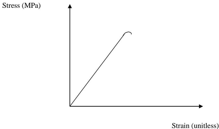
Figure 23 Brittle material
