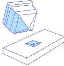
**Figure 34: Vickers hardness test**
