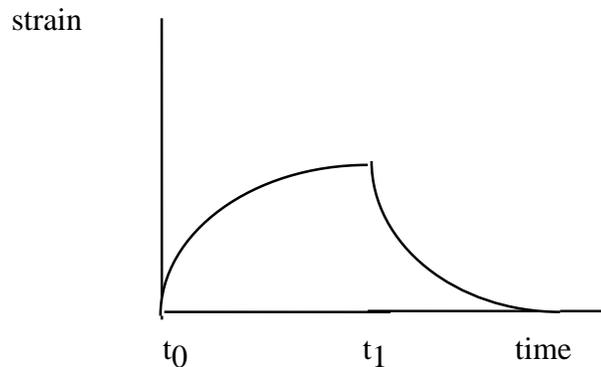
Figure 39: Anelastic behaviour
