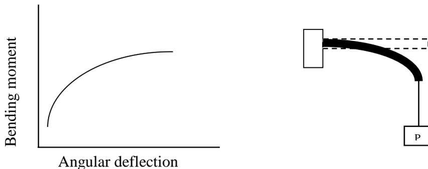
Figure 29: Cantilever bending
