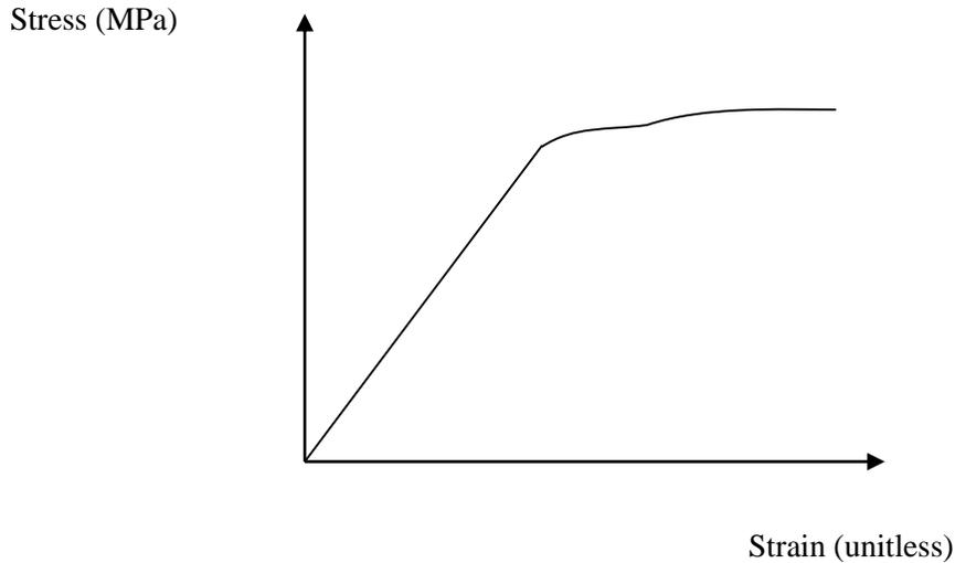
Figure 24 Ductile or malleable material
