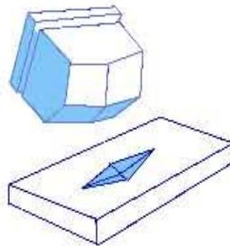
**Figure 33: Knoop hardness test**
