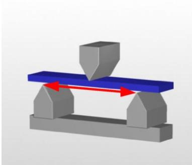
**Significance:** This test is useful in comparing and designing denture base materials and long span bridges. The deformation varies as the cube of the length and the depth or thickness of the beam.
