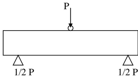
Figure 28 : Measurement of transverse strength
