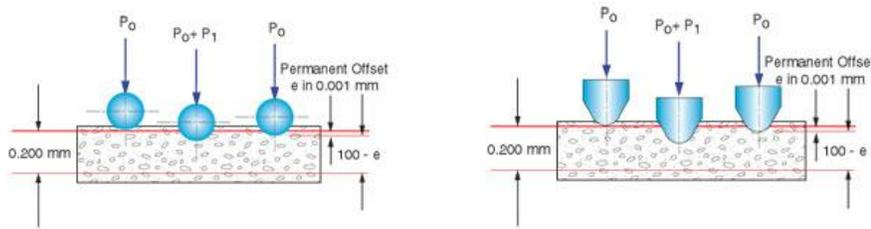
**Figure 35: Rockwell hardness test**
