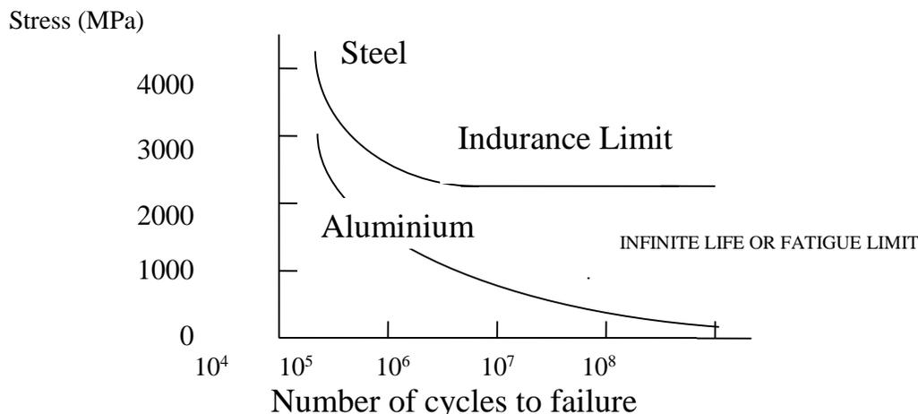
Figure 30 Fatigue strength test.
