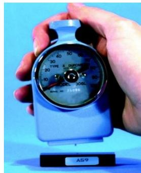
**Figure 36: Shore A test**
