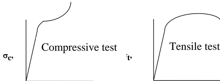
Figure 22b Same slope of the elastic part of both stress strain curves of one material tested under compression and tension
