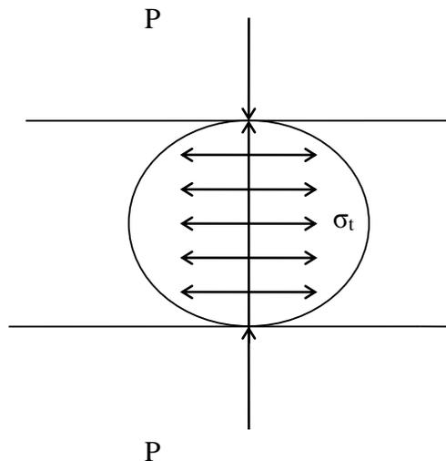
Figure 27 Diametral compression test
